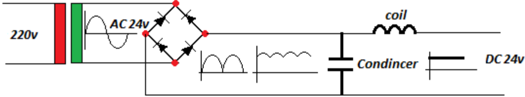
Full Wave Rectifire circuit
